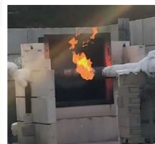
Jet Fire Test Performed according to the ISO 22899-1: 2007
